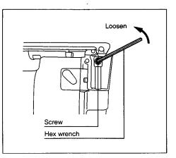
With the blade teeth facing forward, insert the blade into the blade holder as far as it will go. Make sure that the back edge of the blade fits properly in the groove of the roller. Then firmly tighten the screw to secure the blade.
